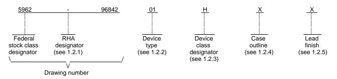
1.2.1 <u>Radiation hardness assurance (RHA) designator</u>. RHA marked devices shall meet the MIL-PRF-38534 specified RHA levels and shall be marked with the appropriate RHA designator. A dash (-) indicates a non-RHA device.
